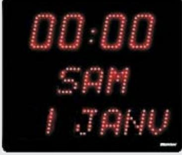
Connect the clock to the mains and apply the power. The clock displays 00:00 SAM 1 JANV while it waits for synchronisation.
