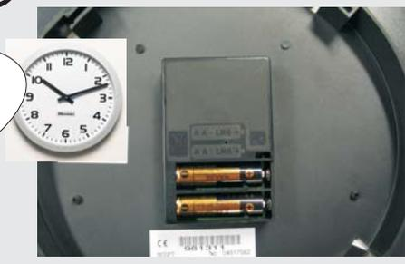
Place yourself where the clock will be installed. Put the batteries in. When inserting the batteries, the hands are set to 4, 8 or 12 h. When the clock will get the DHF signal, it will automatically synchronise.
