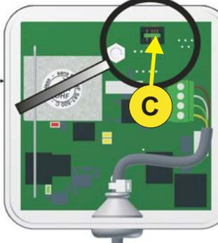
The transmitter is supplied with a dongle. This component includes the parameters required to control of the wireless Melody's and relays. If the transmitter has to be replaced, keep this dongle for the new the transmitter.
