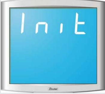
Place yourself where the clock will be installed. Connect the clock to the mains and apply the power. The clock first displays "Init" and then "00:00" while it waits for synchronisation.
