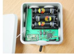
It is recommended to test the HF link before attaching the temperature sensor. Position the plug and the stud before engaging it in the casing. The sensor must imperatively be pointing downwards for obvious waterproofing reasons.
