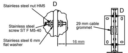
3/ Place the 4 screws (D) at 16 mm. Do not fit the nuts and washers.
