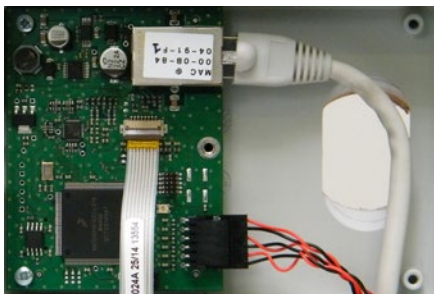
Connection on the circuit board of control box
